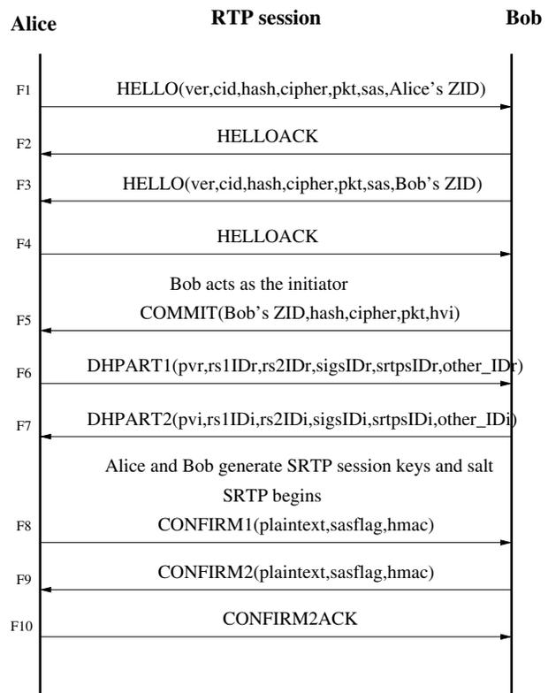
**Figure 3. Establishment of SRTP session key using ZRTP**
